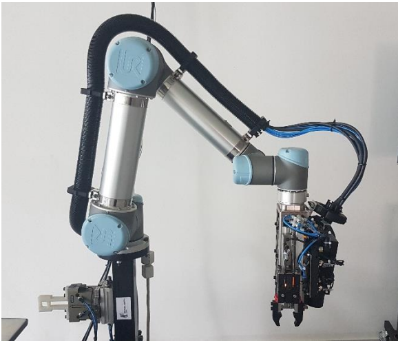
Figure 1: Energy Chain mounted on robot arm
