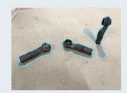
A 2D camera would see these three drive shafts as three different parts. The slightest change in light and shadows would present new contours and confuse the camera even more.
