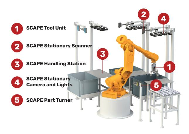
THREE PARTS ARE DELIVERED INTO THE TABLE FIXTURES AVERAGELY EVERY 15-20 SECONDS.
