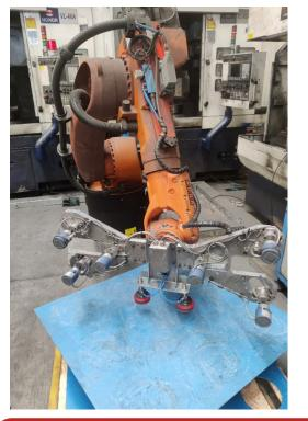
SPEZIALIZED GRIPPER CAN PICK A MULTITUDE OF DIFFERENT SIZES OF DISKS
