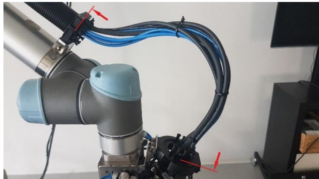
Figure 4: Energy chain with 500-550mm slack
