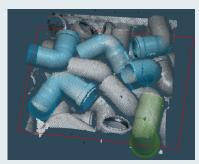
3D vision considers the actual shape rather than a 2D image. The part is initially gripped via the SCAPE 3D Stationary Scanner. Step two is the orientation control via the 2D camera before delivery to the next working station.
