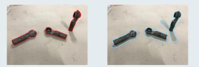
A 2D camera would see these three drive shafts as three different parts. The slightest change in light and shadows would present new contours and confuse the camera even more.
