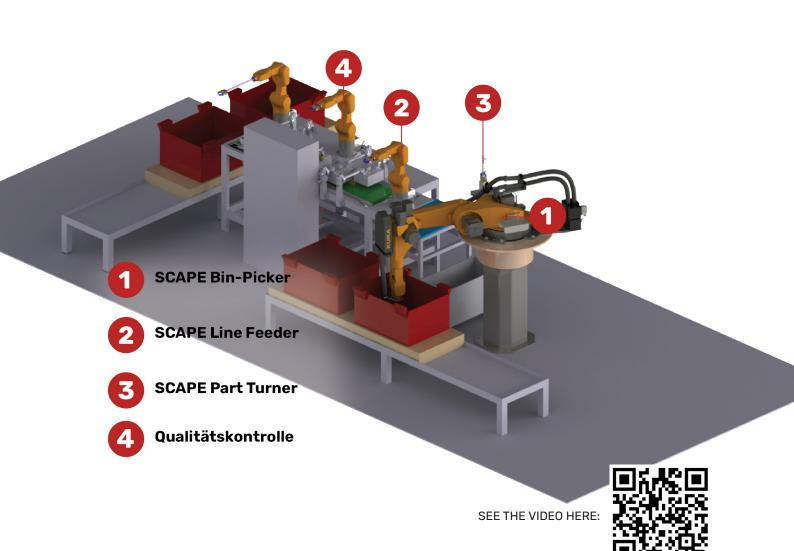
A PART IS DELIVERED INTO THE NEXT PROCESS ON AVERAGE EVERY 10-12 SECONDS.
